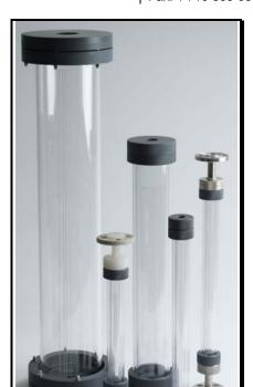
Griffco Borosilicate Glass Calibration Cylinders are designed to enhance the performance of chemical feed systems by providing a verification of the flow rate of the chemical feed pump. Constructed of borosilicate glass and a choice of 8 end cap materials, (PVC, CPVC, PP, PTFE, PVDF, 316SS, Alloy 20, and Hastelloy C) these cylinders are suitable for use with most chemicals. Available in 12 sizes; from 30mL to 20 L.
